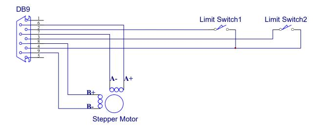
Limit Switch 1 is at the end of the stepper motor. It's the home (zero) position. Limit Switch 2 is at the opposite end of the stepper motor.
